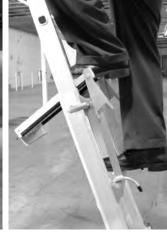
2. Push the Work Platform forward as shown above. Climb the ladder up to the rung above the platform.
