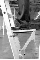
3. Push the Work Platform back with toe until the forward edge of the Work Platform rests securely against the rung. Ensure the Work Platform is securely in position before putting full weight on it.
