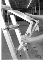
1. Place the wire hooks on the rung below the desired platform height. Place the Work Platform on the rung above the wire hooks. Ensure the Work Platform is securely in position before use.
