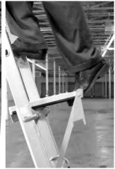
4. When finished using the Work Platform, step to rung above the Work Platform and push the Work Platform forward with toe. Safely step down through Work Platform.
