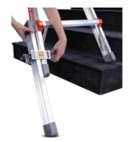
2. Slide the H-bracket onto the outer ladder leg as close to the ladder foot as possible. Insert clamp into the H-bracket and securely tighten. If the angles are not the same, remove leg clamp and rotate the channel assembly 180 degrees, and then replace leg clamp.
